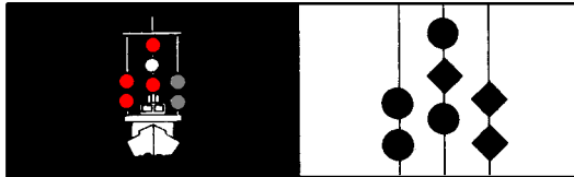
VESSEL ENGAGED IN DREDGING OR UNDERWAY OPERATIONS WHEN RESTRICTED IN ITS ABILITY TO MANEUVER; SHOWING CLEAR AND OBSTRUCTED SIDE.
