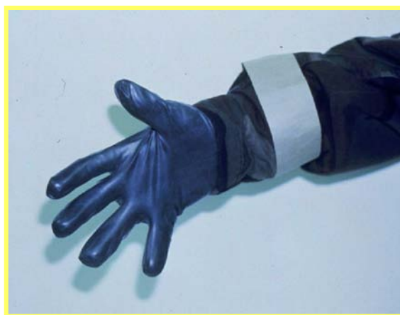
Figure 2-8. M9 Chemical Agent Detection Paper.
