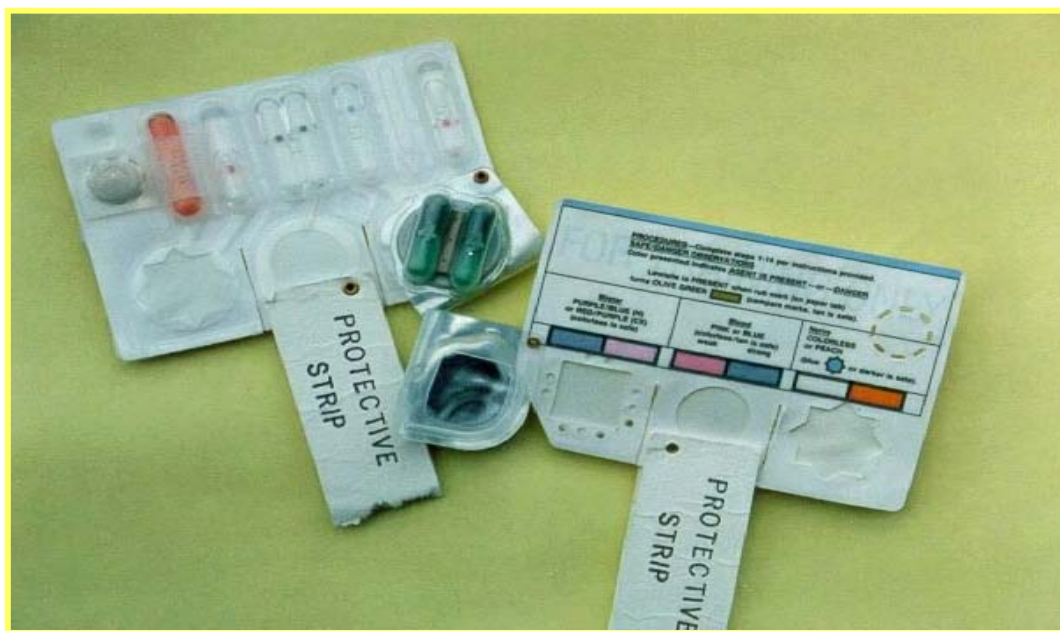
Figure 2-9. M256A1 detector kit.
