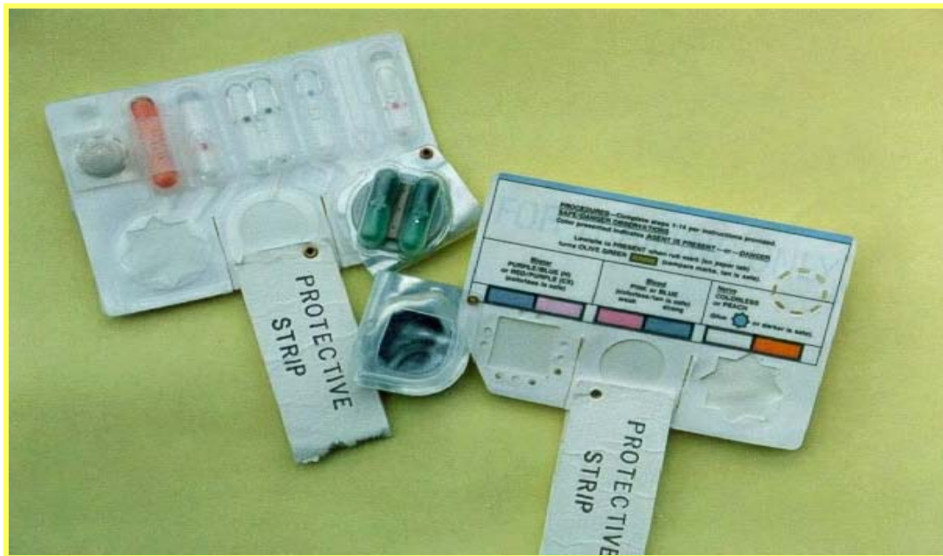
Figure 2-9. M256A1 detector kit.
