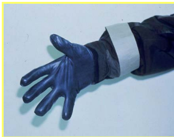
Figure 2-8. M9 Chemical Agent Detection Paper.
